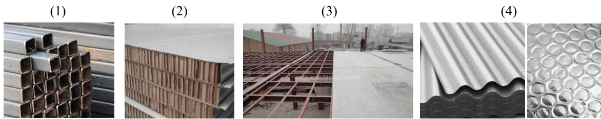
Figure 11:(1) M.S. pipe for the frame, (2) Honeycomb board wall panelling, (3) cement sheet for the floor, and (4) G.I. Sheet with aluminium bubble wrap for insulation
