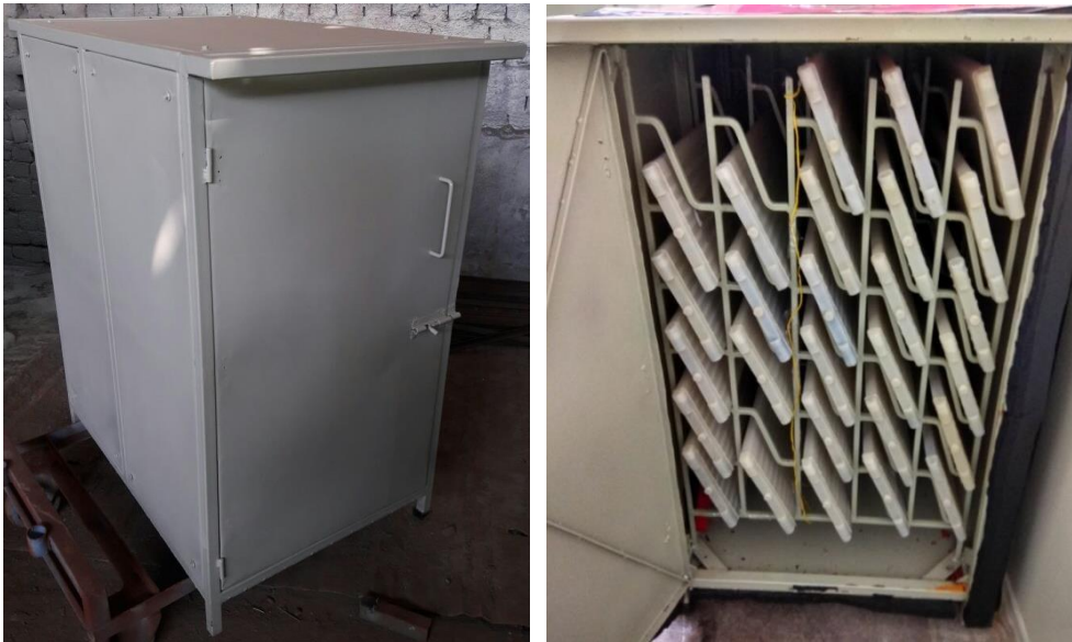
Figure 2: (L) PCM air HX closed view (R) Stacking of the HDPE extruded panels inside HX open view
