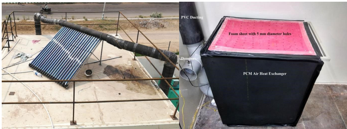
Figure 3: (L) ETC solar collector system with ducting (R) PCM air HX with Nitrile rubber foam insulation and dampers to switch the air circulation during night-time.
