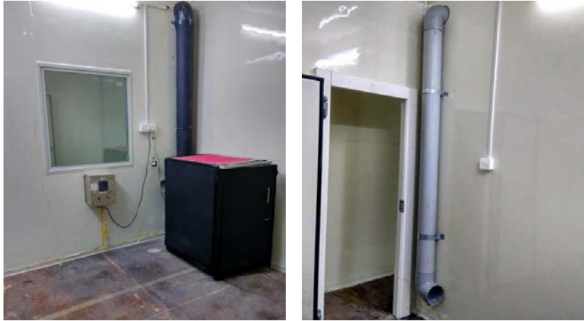
Figure 4: (L) Inside view of the inner room with HX, fan, data logger, and ducting (R) Sucking inlet of the room air
