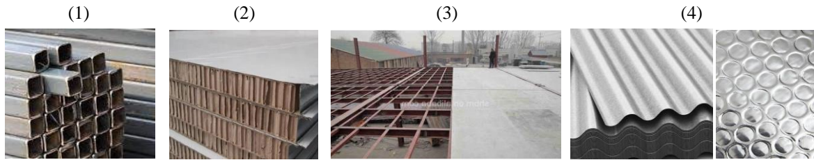
Figure 11:(1) M.S. pipe for the frame, (2) Honeycomb board wall panelling, (3) cement sheet for the floor, and (4) G.I. Sheet with aluminium bubble wrap for insulation
