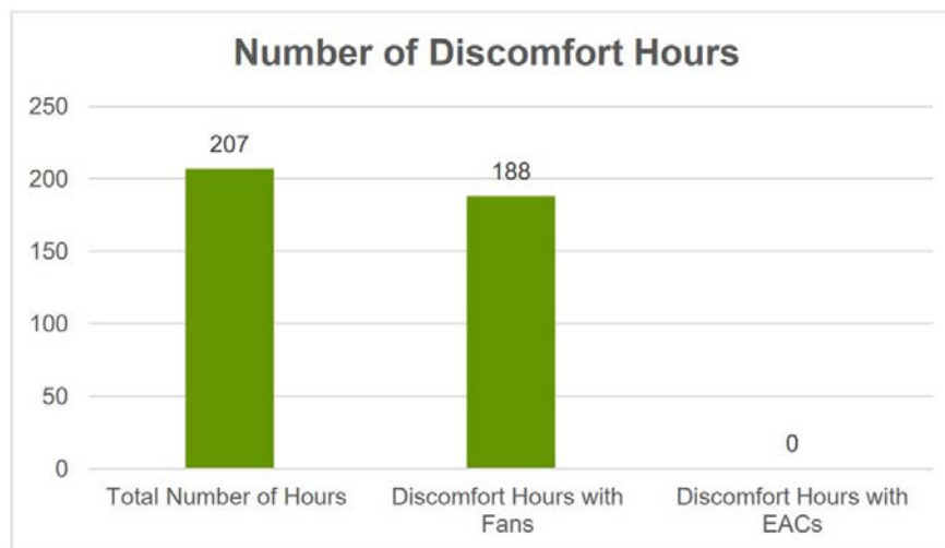
Figure 7: Reduction in Thermal Discomfort Hours Fans vs EACs
