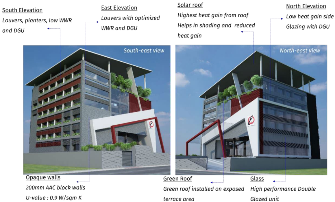
Fig 6: Project is achieving 15 % Savings with the help of Energy efficient building design and selection of appropriate envelope materials
