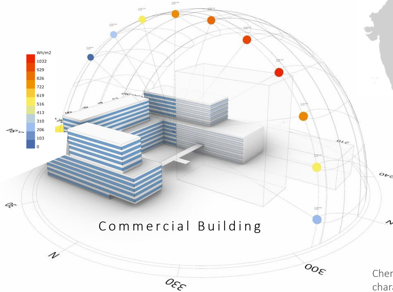
3D Sun-path indicating Solar radiation w.r.t solar position for 21 st July, Sept & Dec (9am-4pm).
