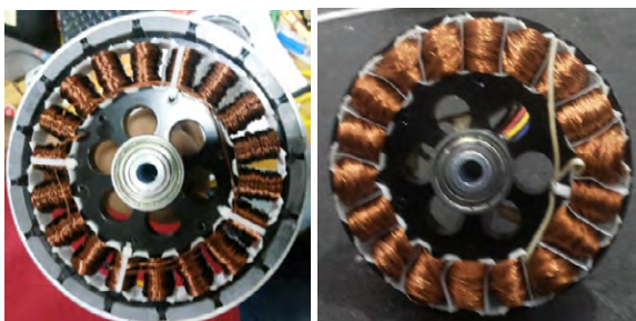
Figure 5: PMBLDCM based fan winding structures of (a) available ceiling fan, and (b) proposed drive
