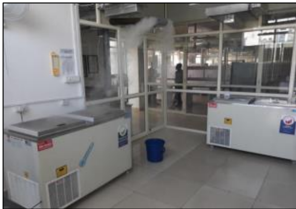
Figure 3: Freezers and coolers with and without PCM under test at an NABL accredited lab in Gurugram.
