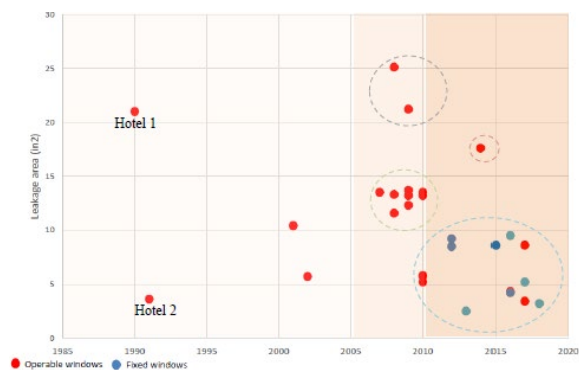
Figure 10 for year of construction of hotel with the leakage area in in 2
