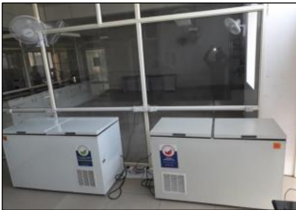
Figure 3: Freezers and coolers with and without PCM under test at an NABL accredited lab in Gurugram.
