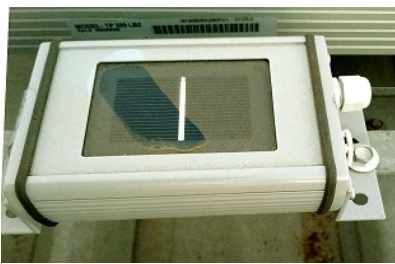
Figure 4: Soiling on irradiation sensor leads to error in performance monitoring of power plant
