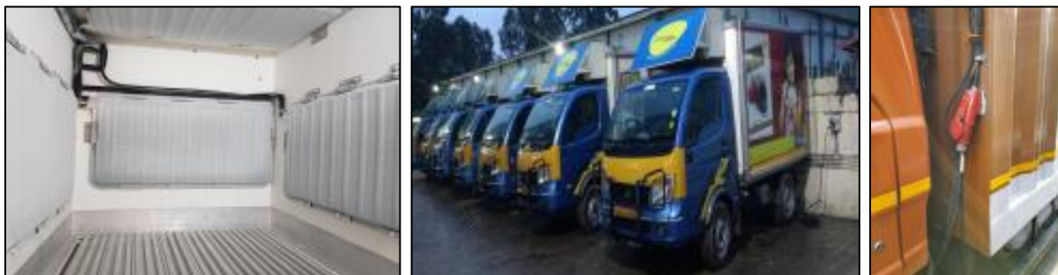
Figure 4: (a) PCM filled metallic plates mounted in insulated reefer trucks; (b) Trucks on standby mode while PCM is charging; (c) Compressor power port for charging the PCM plates.
