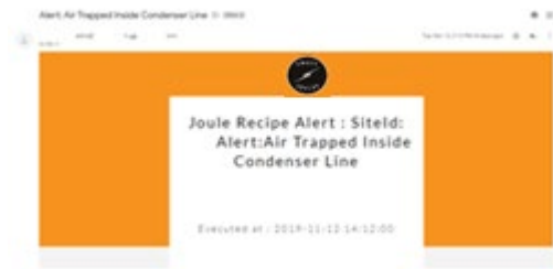
Figure 6: Alert created by Joule Recipe about less flow in the condenser line (preventive maintenance)
