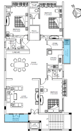
Figure 7: Second floor plan for Project 3 (G+1 storey)
