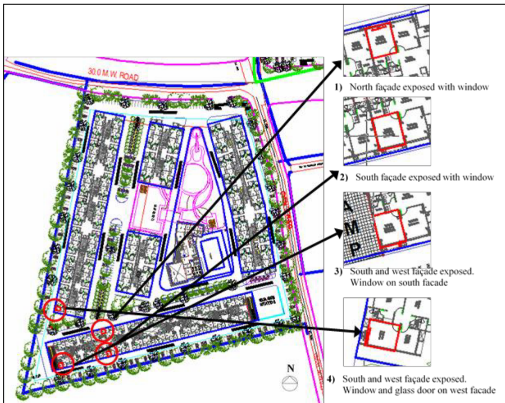
Figure 2: Site plan of Project 1, Indore. The 4 bedrooms selected for simulation are marked
